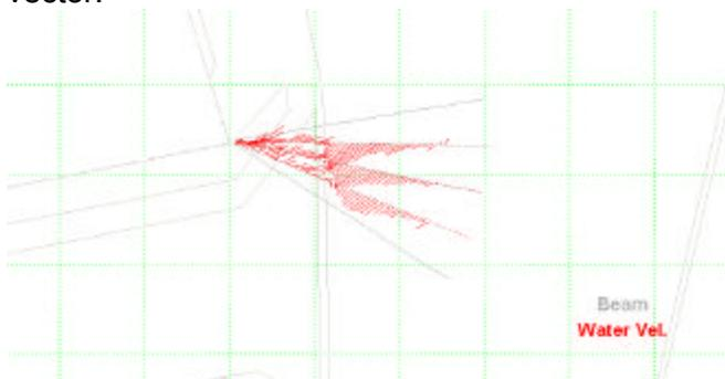
*VISEA-H gives velocity data based on three combinations of the beam data.*
